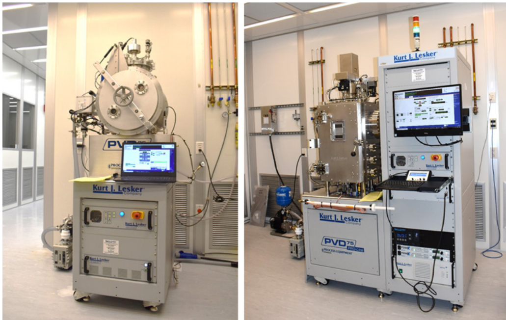
Photos of the Nano36 thermal evaporator (left) and PVD75 e-beam and sputtering system (right).
