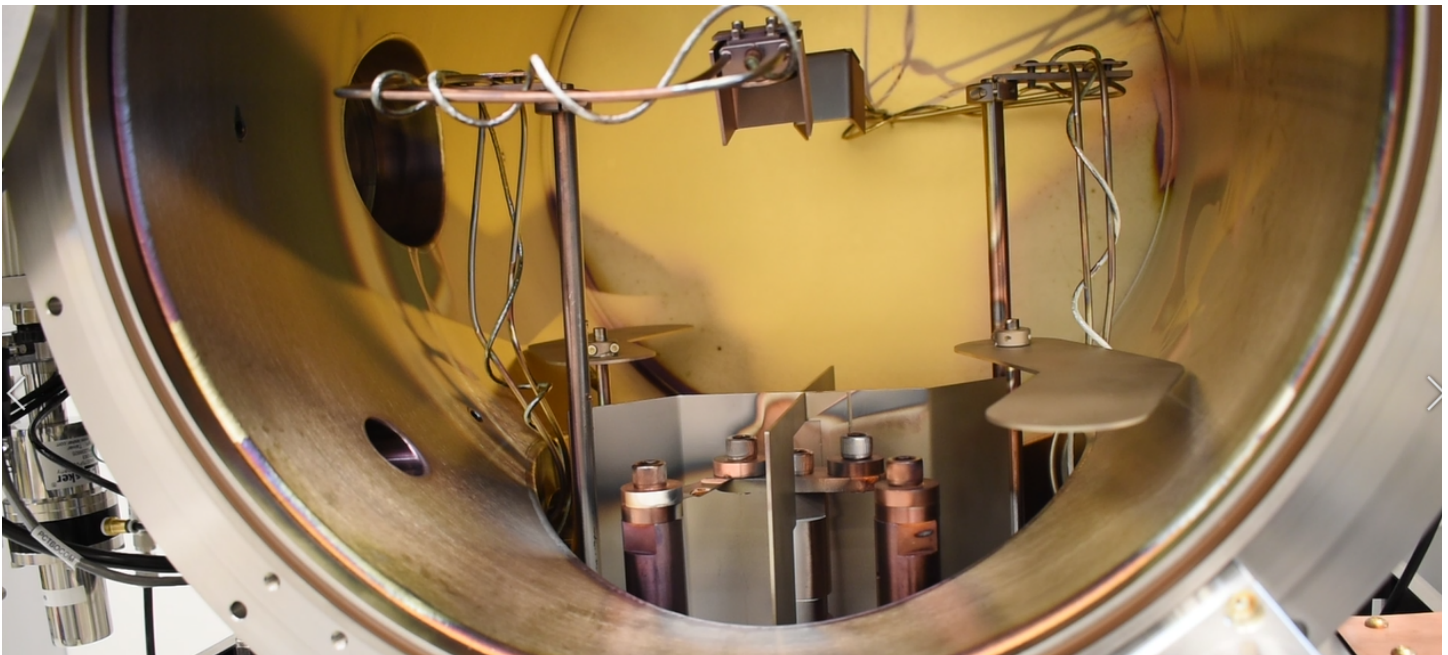
Inside view of the PVD75 showing the sample plate, the e-beam source, the sputtering guns, and QCM.
