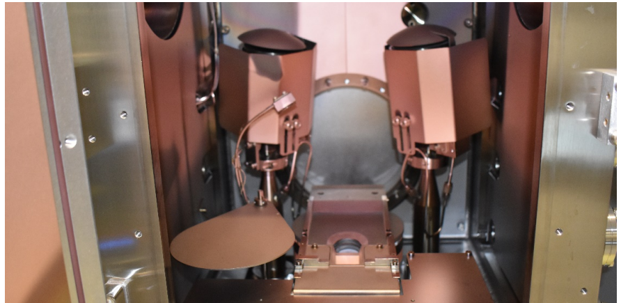
Inside view of the PVD75 showing the sample plate, the e-beam source, the sputtering guns, and QCM.
